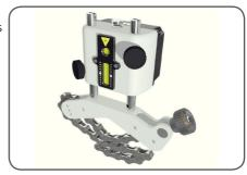
Use the extension chain for shafts > 0150 mm (> 06.0 inch). Press both halves of the link connector together and lock in place by pulling the chain taut.
